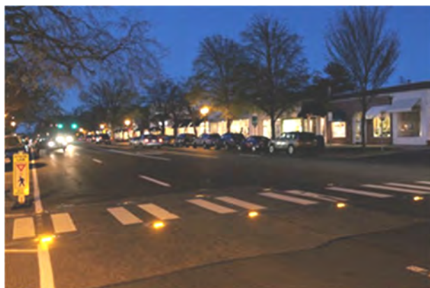
Flashing pavement lights increase pedestrian safety during times of low light.
