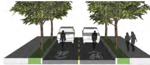
A simple sharrow stencil can be easily applied to roadways to caution drivers of bicyclists.
