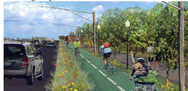
Landscaped buffer between drive lane and bike lane
